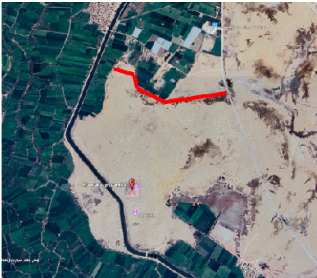
Fig.2 Hawara - drainage line to block subsurface irrigation water
